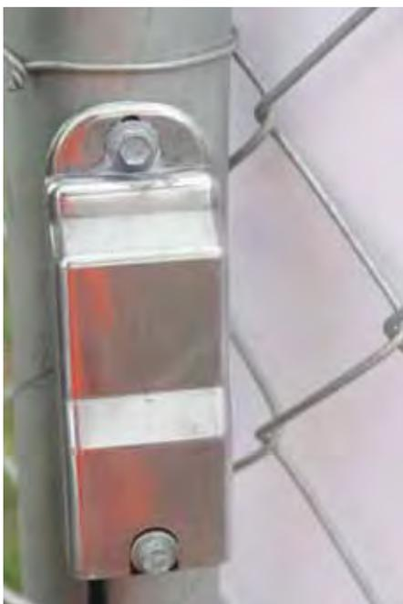
An important feature of the D21 sensor is the alarm processing software which rejects environmental conditions such as change in temperature or disturbances caused by wind and rain. Detection parameters can be defined remotely to achieve the best balance between probability of detection and nuisance alarms.
